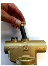
This assembly do not need any specifi sealant; maximum assembly torque: 15 Nm.
